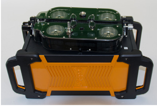
Figure 6–10 Securing drive belt protective covers with bolts
