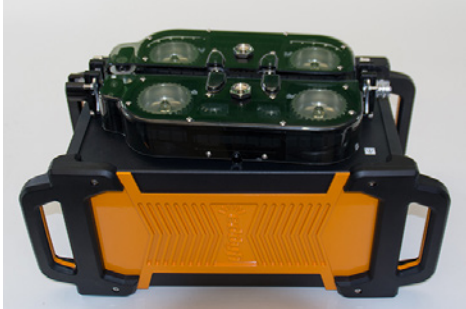
Figure 6-1 Placing the Probot on its side
