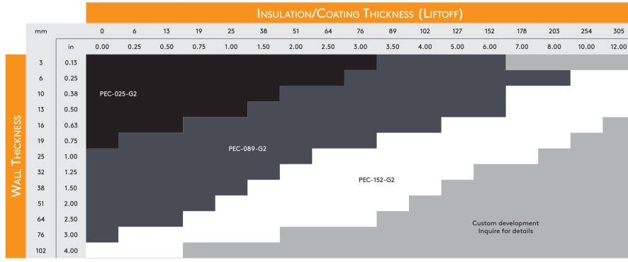
We recommend using the PEC-GS-089-G2 in applications on galvanized steel (GS) weather jackets. If you use other standard probes over GS weather jackets, add 40 mm (1.5 in) liftoff for every 0.5 mm (0.020 in) of GS.
