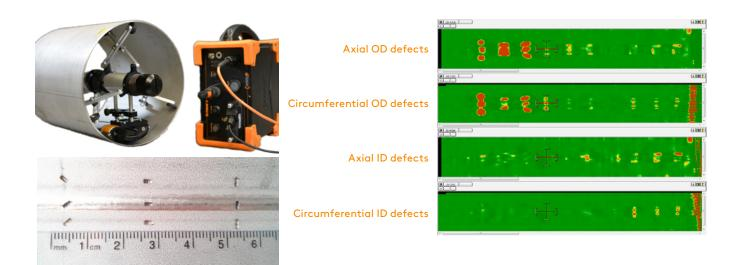
simple to locate defects along a weld's length.
