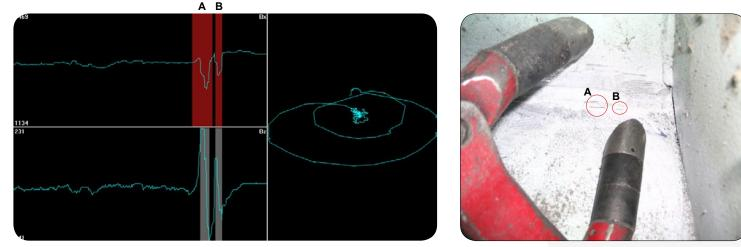
Thames Bridge, built in 1867: ACFM<sup>®</sup> signals from 2 defects on a bridge weld (left) with MPI indications from the same defects (right). Defect **A** was 20 mm long by 3.9 mm deep; defect **B** was 10 mm long by 3.0mm deep.
