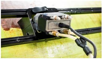
The phased array configuration utilizes a unique water box to create a water-column concept that eliminates the need for a wedge, thus providing the benefits of improved signal consistency, accuracy, and limited dead zone. This concept offers enhanced surface conformity and improved coupling.
